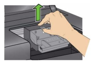
6. Lift the used printhead out of the carriage.
