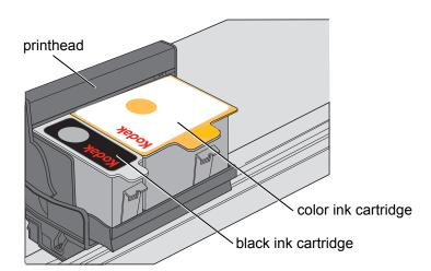
3. Pinch the latch on the ink cartridge and lift it out of the printhead.
