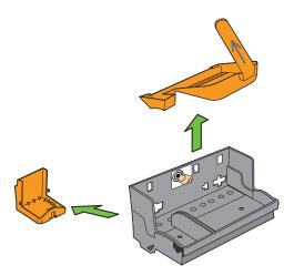
9. Place the new printhead into the carriage. Insert it at the angle shown.
