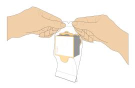
IMPORTANT: Insert the ink cartridge into the printhead immediately to prevent the printhead from drying out.
