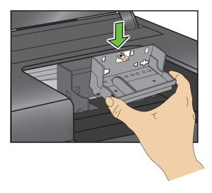
10. Push firmly against the target label of the printhead until you hear a loud snap.
